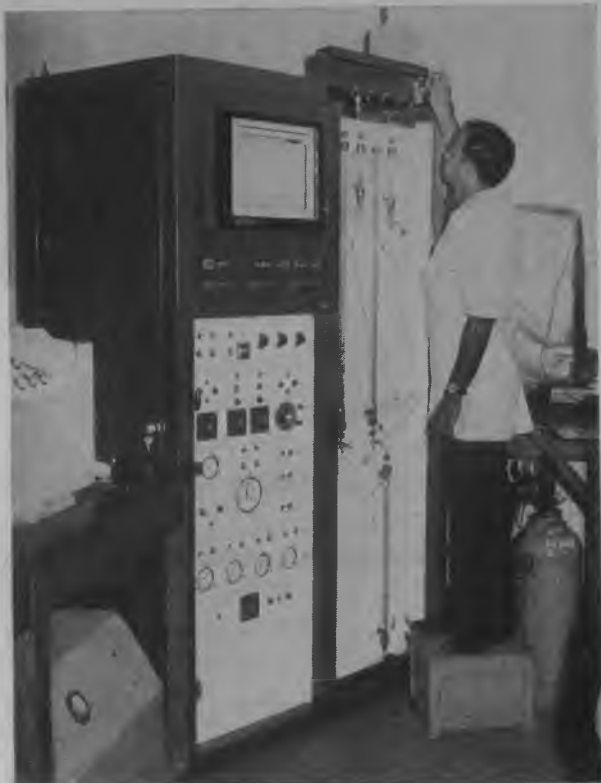
Automatic amino acid analyser (Centre of Advanced Study in Biochemistry, Indian Institute of Science)
