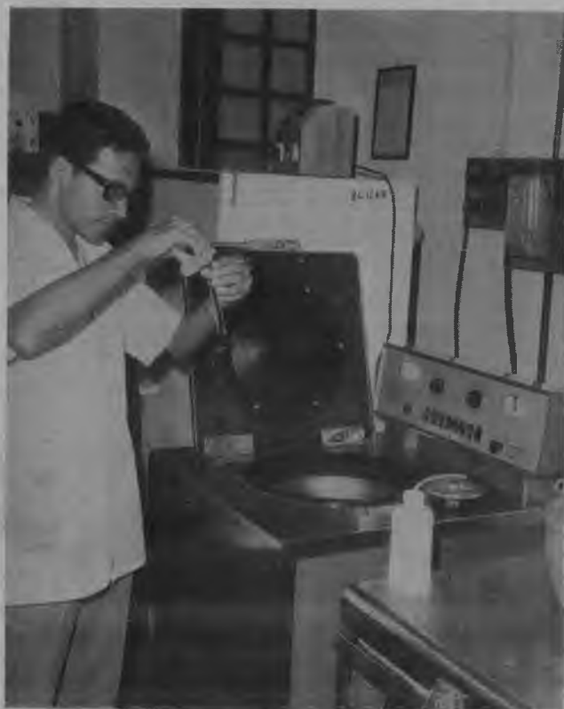
Refrigerated centrifuge (Centre of Advanced Study in Biochemistry, Indian Institute of Science)
