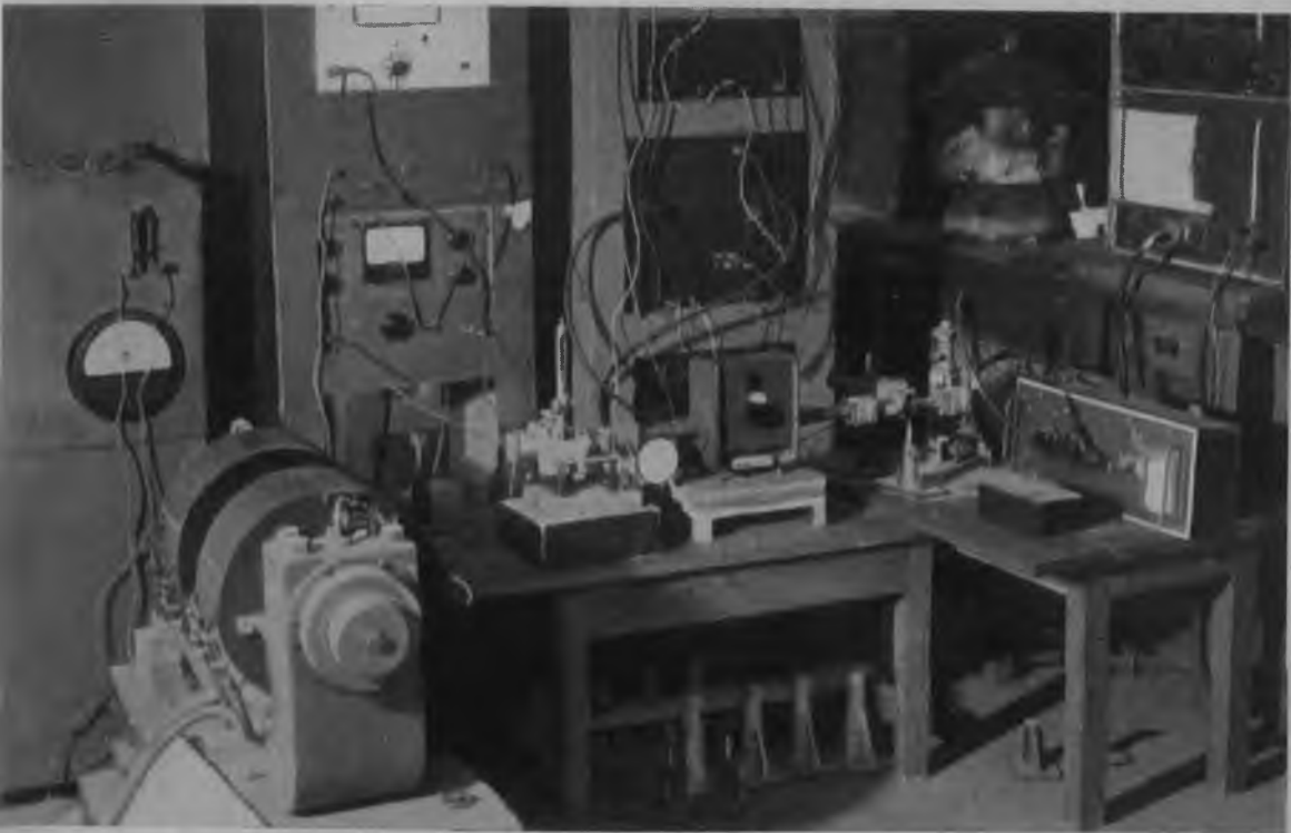
Microwave bridge for the study of semiconductors and artificial dielectrics (Centre of Advanced Study in Radiophysics and Electronics, University of Calcutta)
