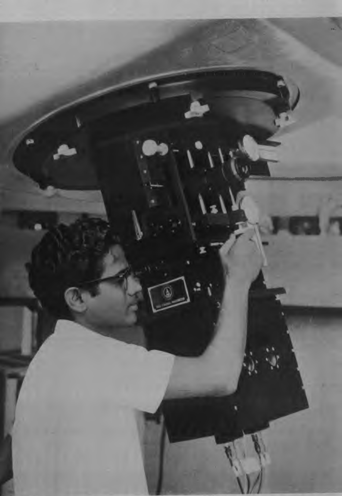
Dual channel photoelectric photometer attached to the cassegrain focus of the 48-inch telescope (Centre of Advanced Study in Astronomy, Osmania University)
