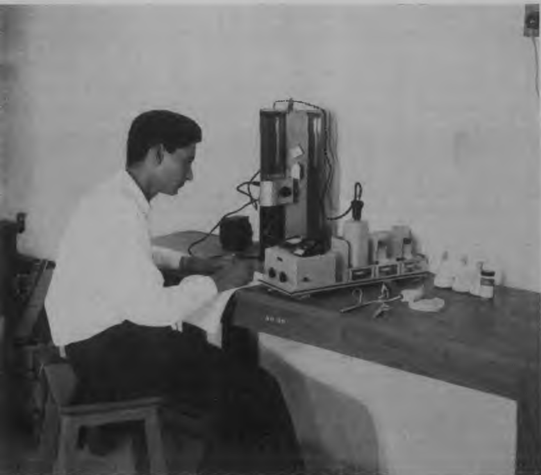
Differential thermal analysis of clay minerals (Centre of Advanced Study in Geology, Saugar University)
