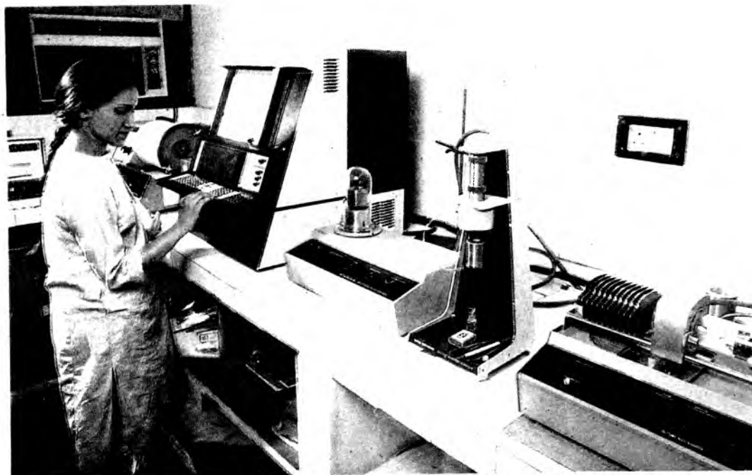
Centre for Materials Science & Technology, IIT, New Delhi—Thermal analyser in materials research.
