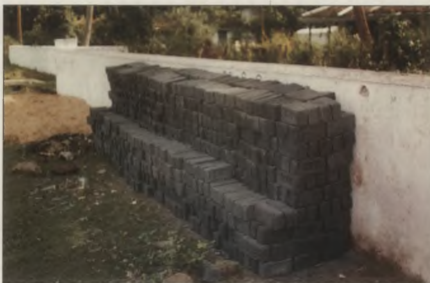
Fly-ash bricks are used for construction of toilets in Orissa.
