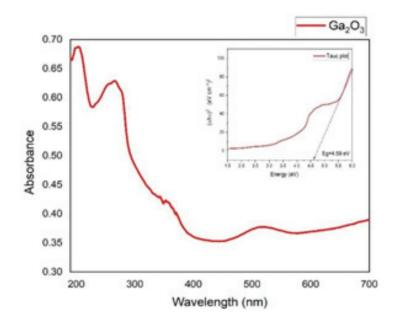
Figure 3. UV-Visible absorption spectra of pure Ga2O3
