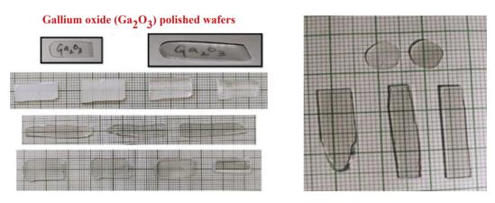
Fig 2 Cut and processed Gallium oxide single crystal wafers
