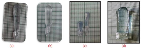
Figure 1. (a) Pure, (b) Sn- doped, (c) Si doped (0.1 and 0.2 %) and (d) Si doped (0.05 %) β- Ga2O3
