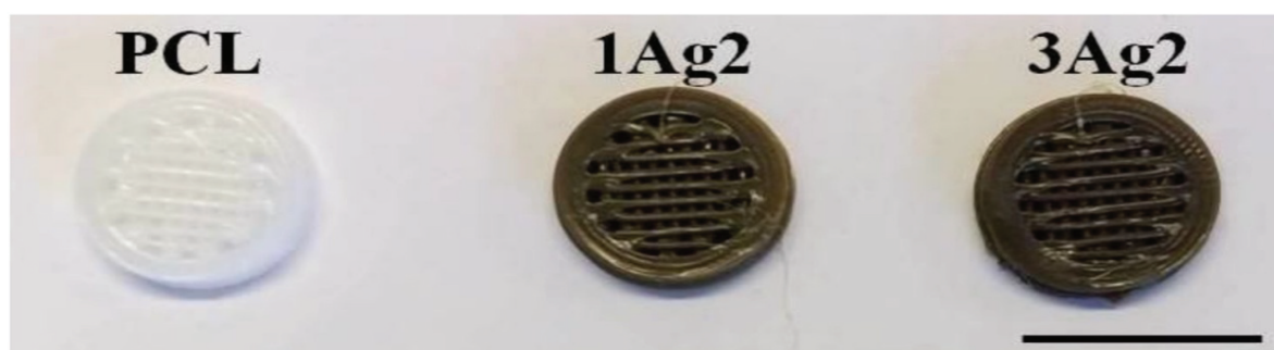
Fig. 3D printed polycaprolactone scaffolds (scale bar denotes 1 cm).
