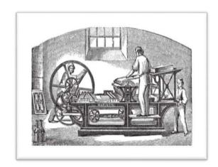
A **printing press** is a mechanical device for applying pressure to an <u>inked</u> surface resting upon a <u>print</u>
