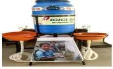
innovative device of multi-tap water source at the tube-well point or at the pipe source point has been introduced with little expenditure of a plastic pipe, few taps and if required a rubber pipe. With the help of this
