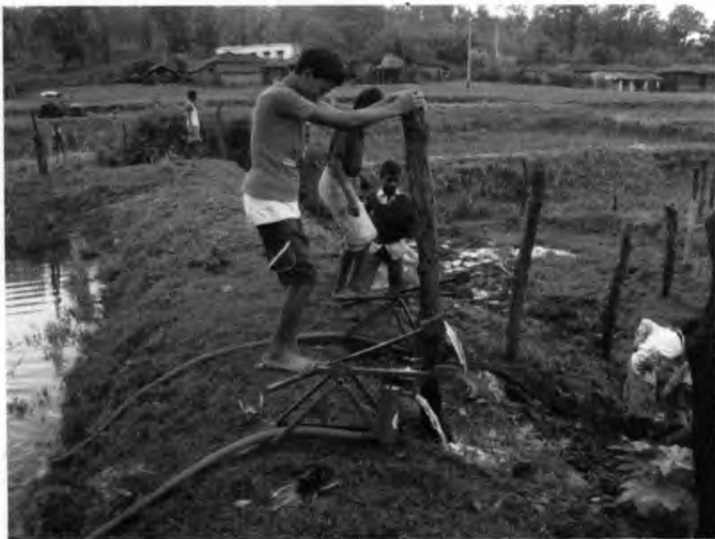
Treadle Pump- A Farmer Pocket Friendly Lifting Device
