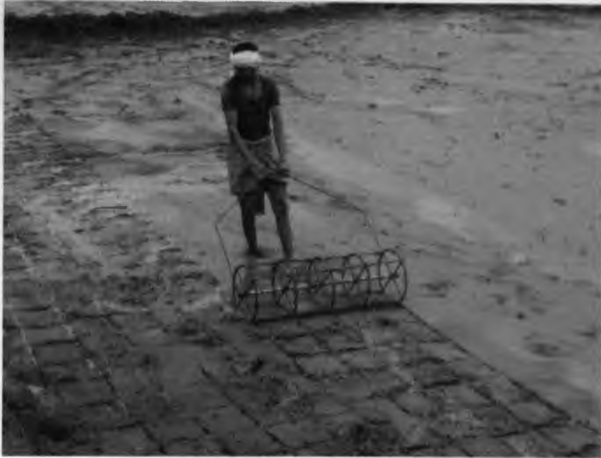
Locally made Marker, for SRI
